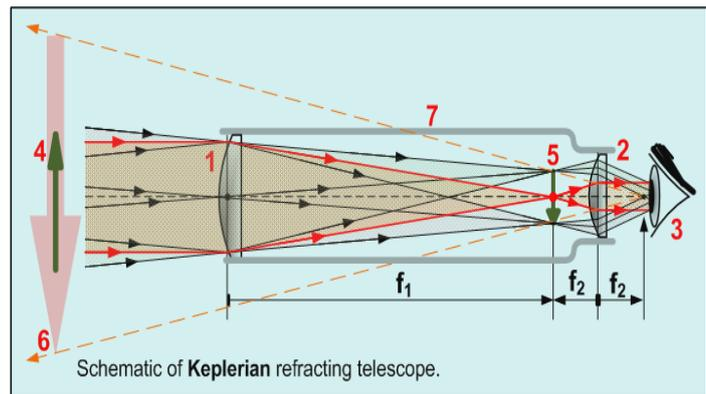
The objective in a refracting telescope refracts or bends light. This refraction causes parallel light rays to converge at a focal point; while those not parallel converge upon a focal plane. The telescope converts a bundle of parallel rays to make an angle  $\alpha$ , with the optical axis to a second parallel bundle with angle  $\beta$ . The ratio  $\beta/\alpha$  is called the angular magnification. It equals the ratio between the retinal image sizes obtained with and without the telescope.
