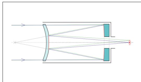
**Schmidt–Cassegrain telescopes:** Schmidt-Cassegrain telescopes are one of the most popular commercial designs on the amateur astronomical market. The design replaces the Schmidt Camera film holder with a Cassegrain secondary mirror making a folded optical path with a long focal length and a narrow field of view.
